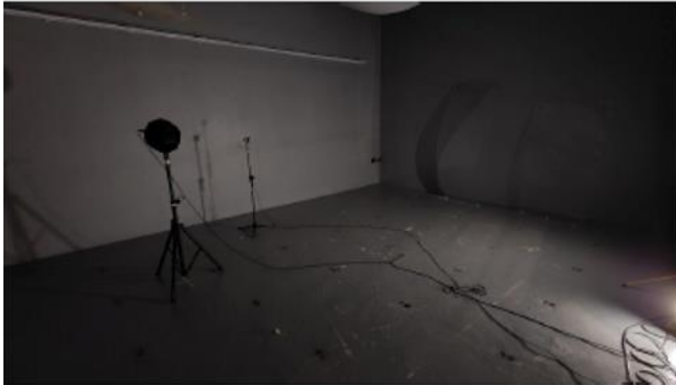
Figure 1: reverberation chamber assembly with source only
